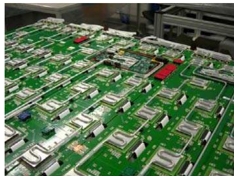
Figure 2: Cooling pipes glued to readout boards.
