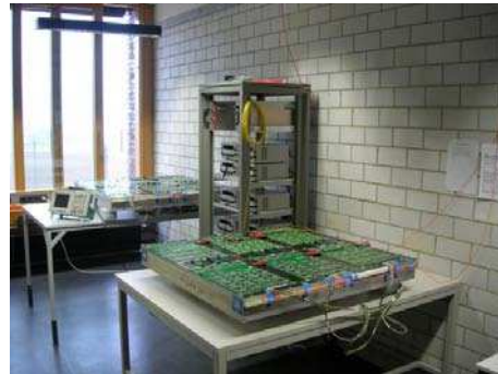
Figure 1: Electronic test stands for the ALICE TRD chambers with pulser and low voltage support.
