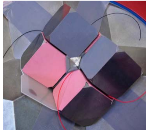
Figure 3.2: The pressure cell (with two thermocouples) is surrounded by six (of eight) WC-cubes.
