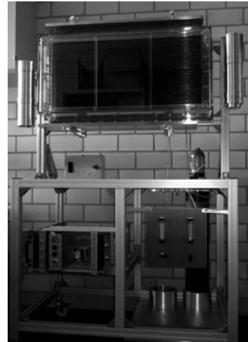
Figure 2: Photo of the spark chamber at the IKF lab. The brass plates, gas volume, Plexiglas cover and trigger detectors can be seen at the top. At the lower left, the electronics is shown. The gas system with flow meters and gas bottles can be found at the lower right.
