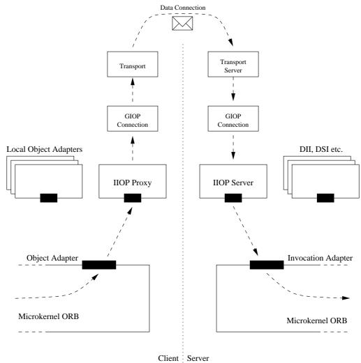
Figure 5.2: Remote invocation with a microkernel ORB
