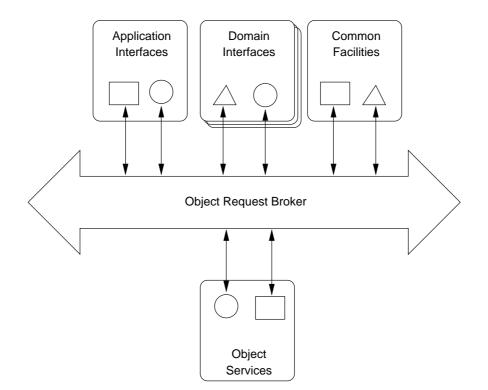
Figure 3.1: The Object Management Architecture Reference Model
