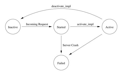
Figure 5.8: Implementation States according to the POA Mediator
