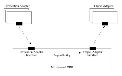
Figure 5.1: The MICO microkernel ORB
