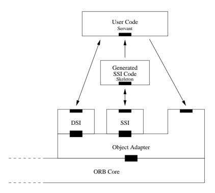
Figure 4.1: Server-side view of the ORB
