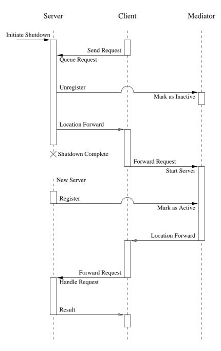
Figure 5.9: Handling of requests during server shutdown
