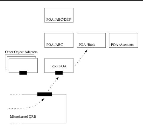
Figure 5.3: Only the Root POA is registered with the MICO ORB
