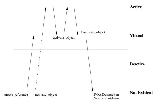
Figure 4.8: Lifecycle for transient objects using the POA
