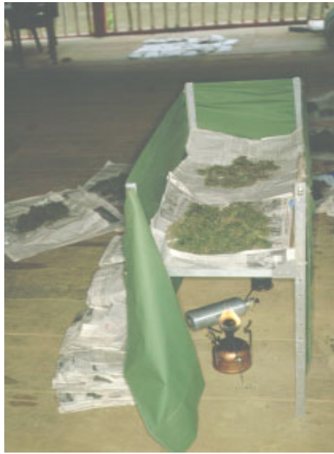
Fig. I.3: Dryer from fig. I.1 in action, front removed to show the stoves (Irangi, Congo, former fieldstation of King Leopold II).
