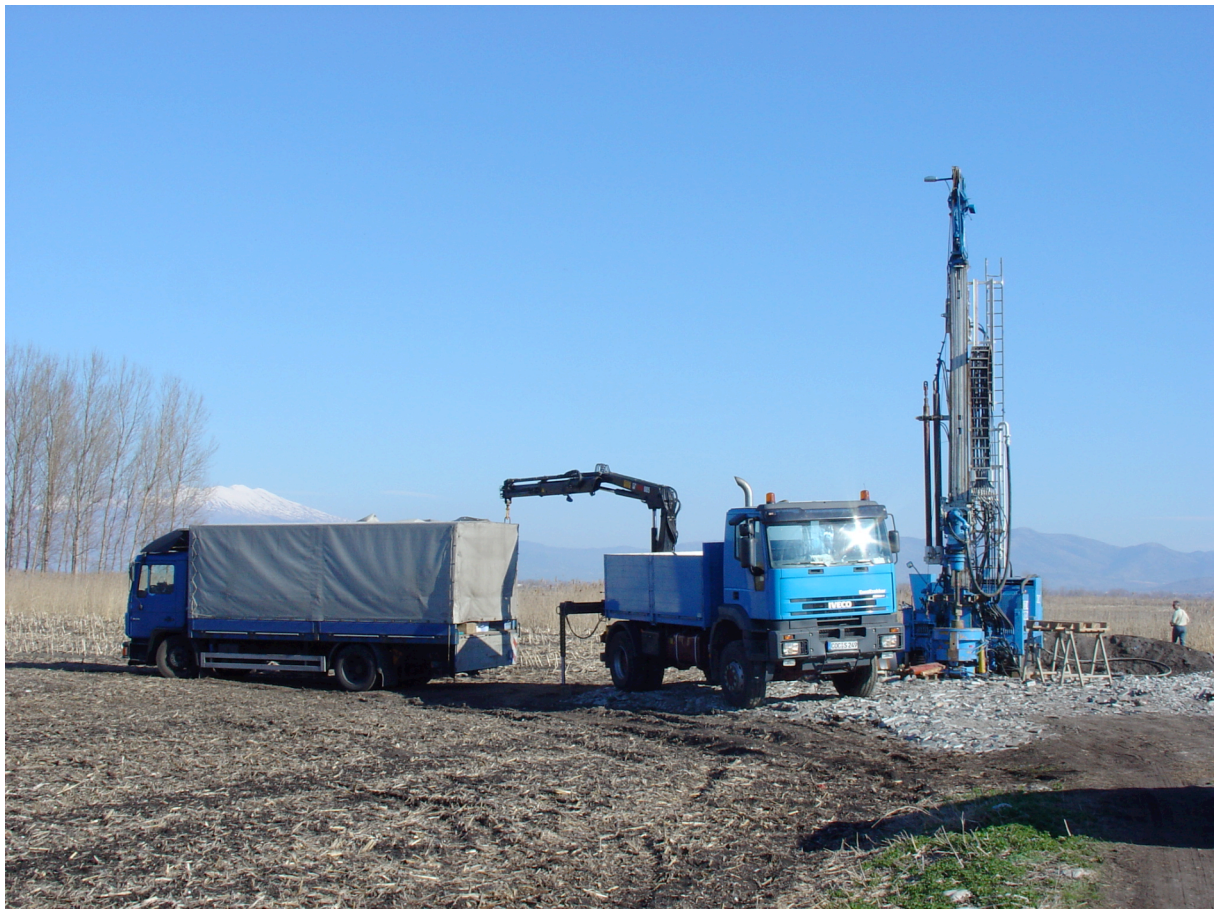
Fig. 2. Drilling rig WIRTH Eco1 used for drilling in the Drama Basin. The Phalakro mountain range (2232 m a.s.l.), which borders the Drama Basin to the northeast, is visible in the background. Photograph by Ulrich C. Müller.
