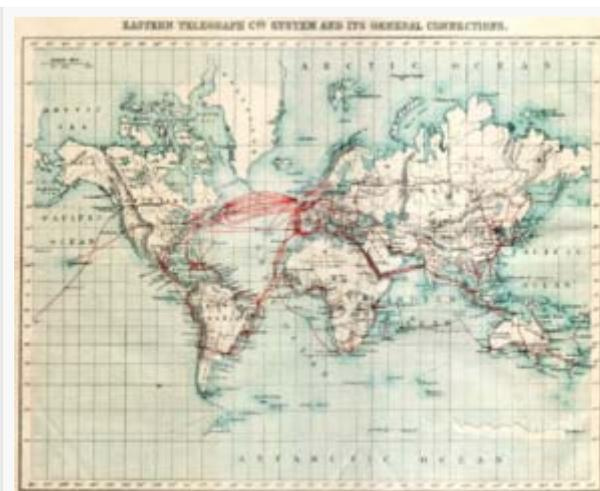
The Eastern Telegraph Co.: System and its general connections. Chart of submarine telegraph cable routes, showing the global reach of telecommunications at the beginning of the 20th century (A.B.C. Telegraphic Code 5th Edition)
