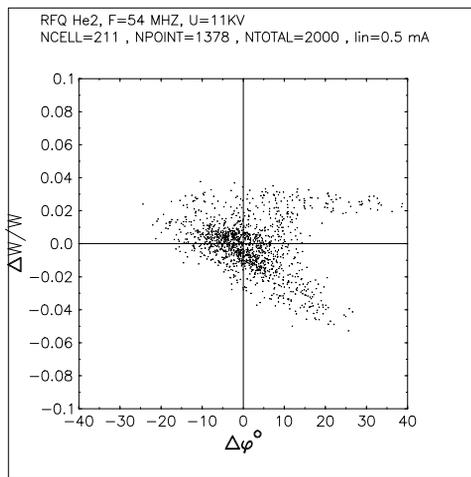
Figure 7: PARMTEQ simulation of the phase width at the beam crossing point.
