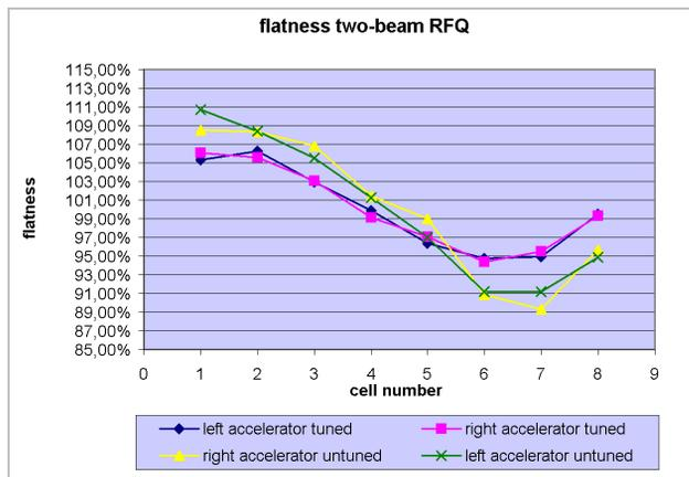
Figure 3: Longitudinal voltage distribution in the RFQ.
