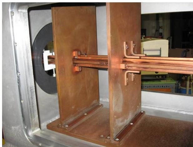
Figure 4: Small tuning angles as additional capacity for a better voltage symmetry.
