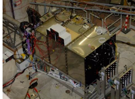
Figure 2.11: Photograph of constructed 3 layers of RICH Detector walls under test during CERN beam-time
