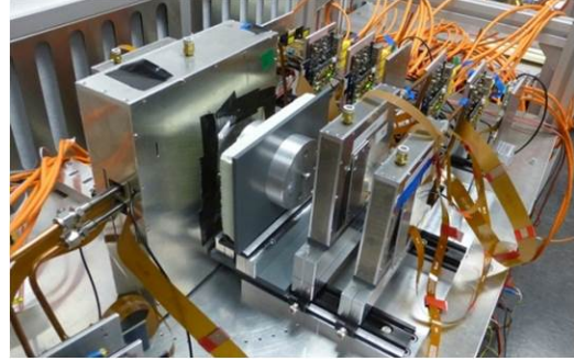
Figure 2.7: A photograph of prototype Micro-Vertex Detectors under test in the laboratory.
