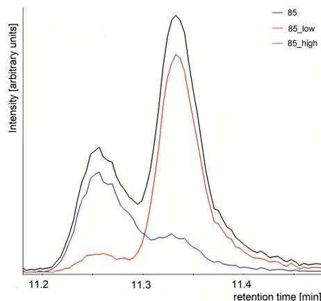
**Figure 5.** A chromatogram of an unidentified hydrocarbon peak (smaller one) eluting slightly earlier than the higher Trichloromethane peak. The nominal mass 85 u (black) shows a double peak. By choosing the lower mass range (84.7 u to 85.0 u; red) a lower signal for the unidentified hydrocarbon peak is observed, and by choosing the higher mass range (85.0 u to 85.3 u, blue) a lower signal for the Trichloromethane peak is observed.
