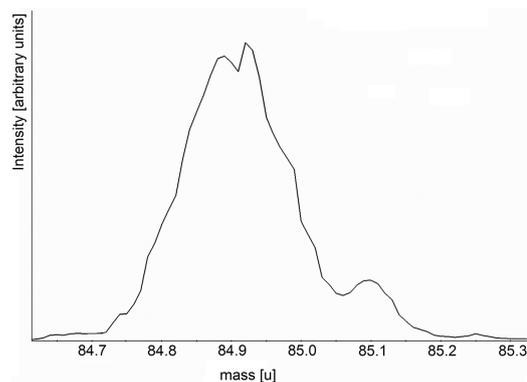
**Figure 4.** So-called 0.01 u mass spectrum of the substance Trichloromethane. Two mass peaks are shown. The higher one by mass 84.9 u is identified as the molecule fragment (CH<sup>35</sup>Cl<sup>37</sup>Cl<sup>+</sup>) and the other one by mass 85.1 u is an unidentified hydrocarbon peak.
