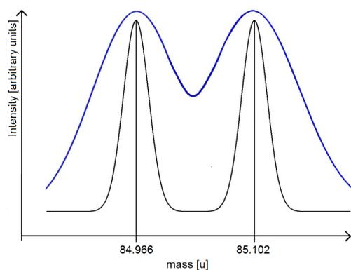
**Figure 3.** Schematic display of two different mass resolutions (blue and black curves). Two signals on masses 84.966 and 85.102 u with equal intensities demonstrate the mass separation with  $R = 600$  (blue curve) and  $R = 3700$  (black curve). Assuming Gaussian peak shapes for the signals,  $R = 3700$  separates both peak by  $8\sigma$  (quantitative separation) and  $R = 600$  separates them by only  $2\sigma$  (qualitative separation).
