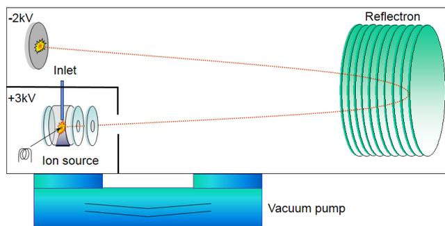
**Figure 2.** Scheme for the direct ion extraction of the Bench TOF-dx direct extraction (five technologies GmbH, G. Horner and P. Schanen, personal communication, 2014). The red dotted line represents a typical ion path.
