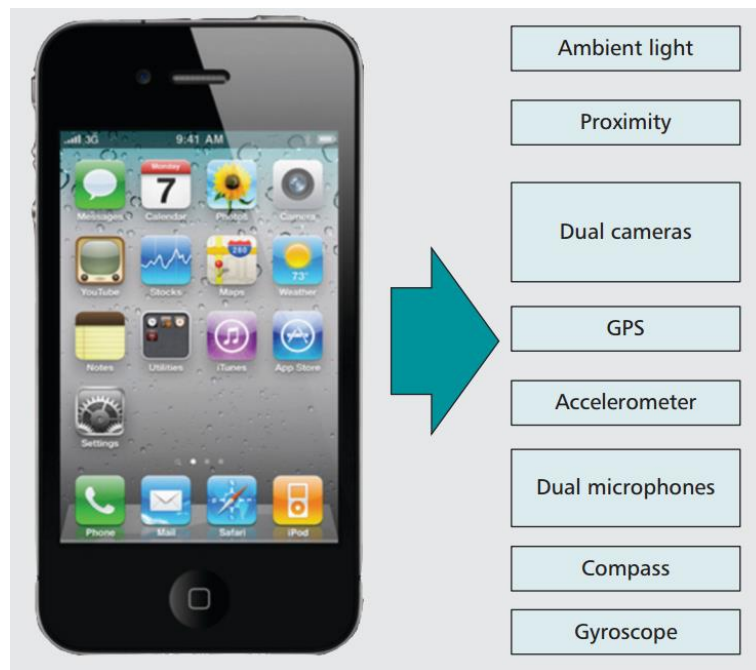
Figure 3.13.: Integrated sensors in the iPhone 4 [LML + 10]
