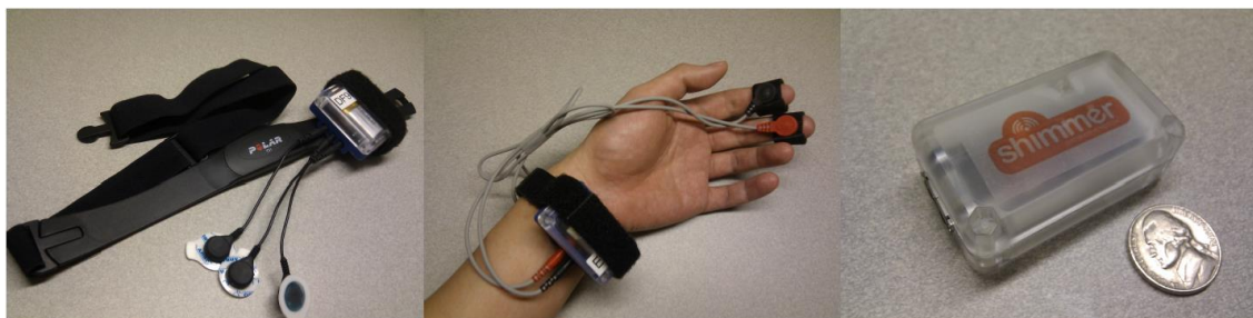
Figure 3.17.: Sensors for measurement of ECG, EDA and Activity used in the study of Sun et al. [SKC + 12]
