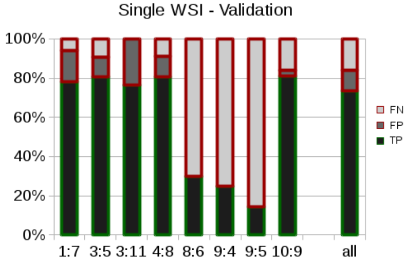
Figure 4.35: Pipeline validation for a single WSI The TPs, FPs, and FNs for a single WSI are plotted. The results are depicted for single tiles and the total result for all tiles. Overall, most cell objects were detected by the pipeline and the amount of FP cell objects is low. The precision and sensitivity are higher than 80 %. But for single tiles the quality of the detection drops down. The three image tiles 8:6, 9:4, and 9:5 have a high amount of FNs. For the three tiles we also observed a low quality of staining. The low intensity of the fuchsin stain is a likely explanation for the high FN-rate.
