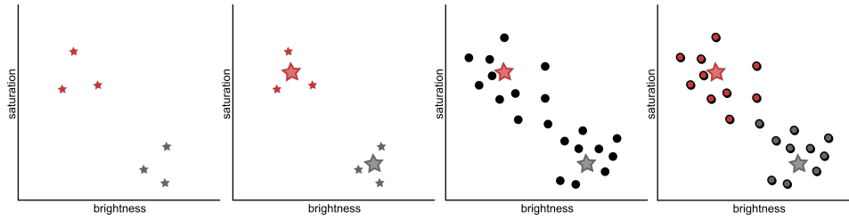
Figure 3.4: Minimum distance to mean clustering The algorithm can be divided into three steps: First an annotated set of training samples is chosen. They are used to calculate the cluster heads in the second step. Third, test samples are classified, by choosing the cluster head with the minimum distance. Here, two pixel descriptors are considered, the saturation and the brightness of the pixel.
