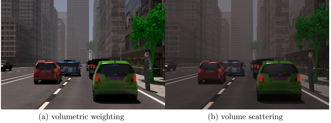
Figure 3.3: Mathematically simplified and physically based Fog effects
