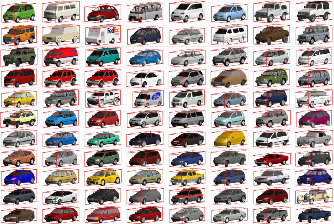
Figure 3.1: A few 3D CAD vehicle models downloaded from Google’s 3D warehouse. These CAD models are used in [23] for 3D object detection.
