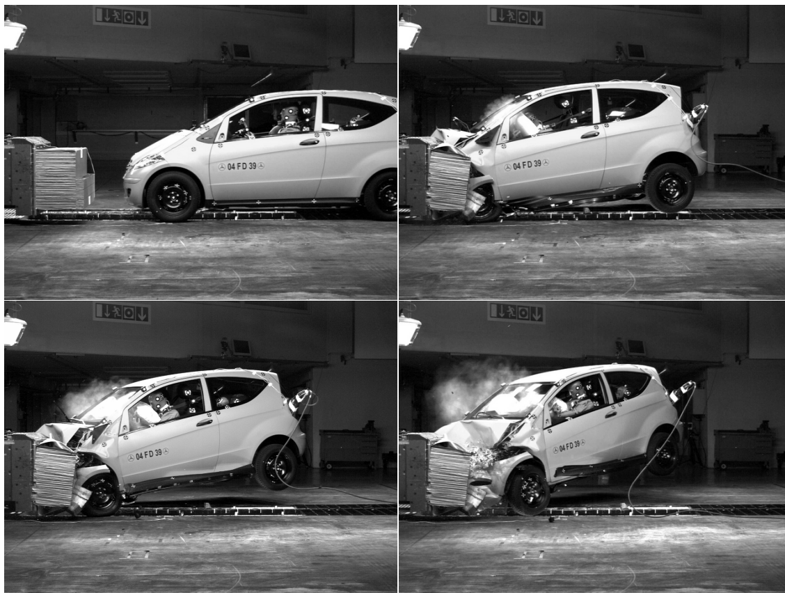
Figure 8.13: Snapshots of the sequence Crash Test . Top-Left and bottom-right images show the first and last frame the sequence. The top-right image shows the moment of deepest airbag penetration. The bottom-left image shows the image at which the head is totally visible once again.
