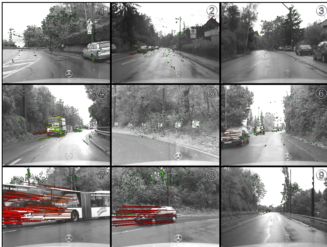
Figure 8.5: Snapshots of the estimated velocity of tracked points for the sequence Curves .
