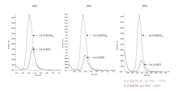
Supplementary Fig. S2. Chromatograms of 14,15-EET in the murine ophthalmic artery. Representative LC-MS/MS chromatogram of 14, 15-EET (in red) compared to deuterated internal standard (in blue). R1- R3: replicate 1-3; n = 5/ replicate. cps: count per second.
