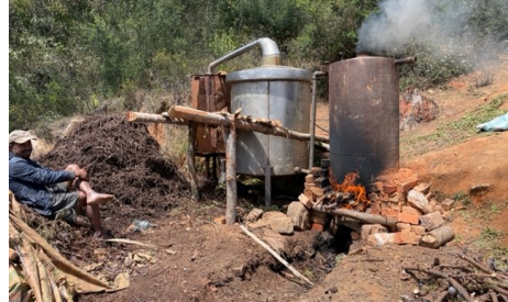
Fragrant Geranium essential oil distillery by the road.
