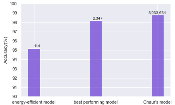
Figure 7: Comparison of the most energy efficient model using the proposed workflow (Model 4), the best performing model (Model 6) and Chaur’s model [24]. The numbers on top of the bars indicate the size of the model with respect to the trainable parameters.
