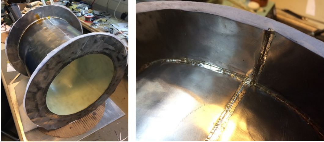
Figure 4.11: Photographs of the CRY-aCCC during the construction. (left) The first screening ring is glued to the inner fiberglass support tube. (right) Close-up view of the soldering connection that has to form a superconducting interface between the lead sheets that is free of any pinholes.
