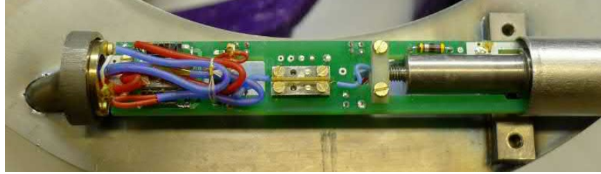
Figure 3.3: SQUID cartridge of a very similar CCC system in operation at CERN. The cartridge encloses the flux transformer and the SQUID sensor, which is protected by an additional shielding can on the right hand side. On the far left the cartridge is connected to the shield enclosing the pick-up coil. Picture taken from [8].
