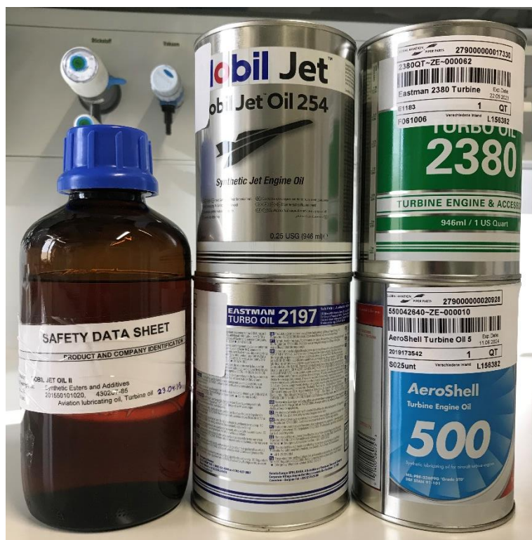
Figure 10. The analysed jet engine oils (Mobil Jet Oil II, Mobil Jet Oil 254, AeroShell 500, Eastman Turbo Oil 2197 and Eastman Turbo Oil 2380).
