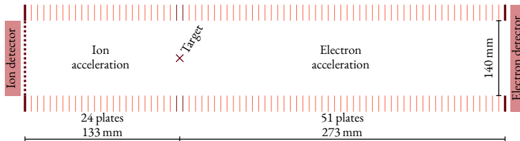
FIGURE 8.13: Sketch of the spectrometer of the beam time in August 2018 at beam line ID31 at the ESRF, Grenoble. Note that two target plates instead of one were used to ensure that the synchrotron beam does not collide with the spectrometer plates.
