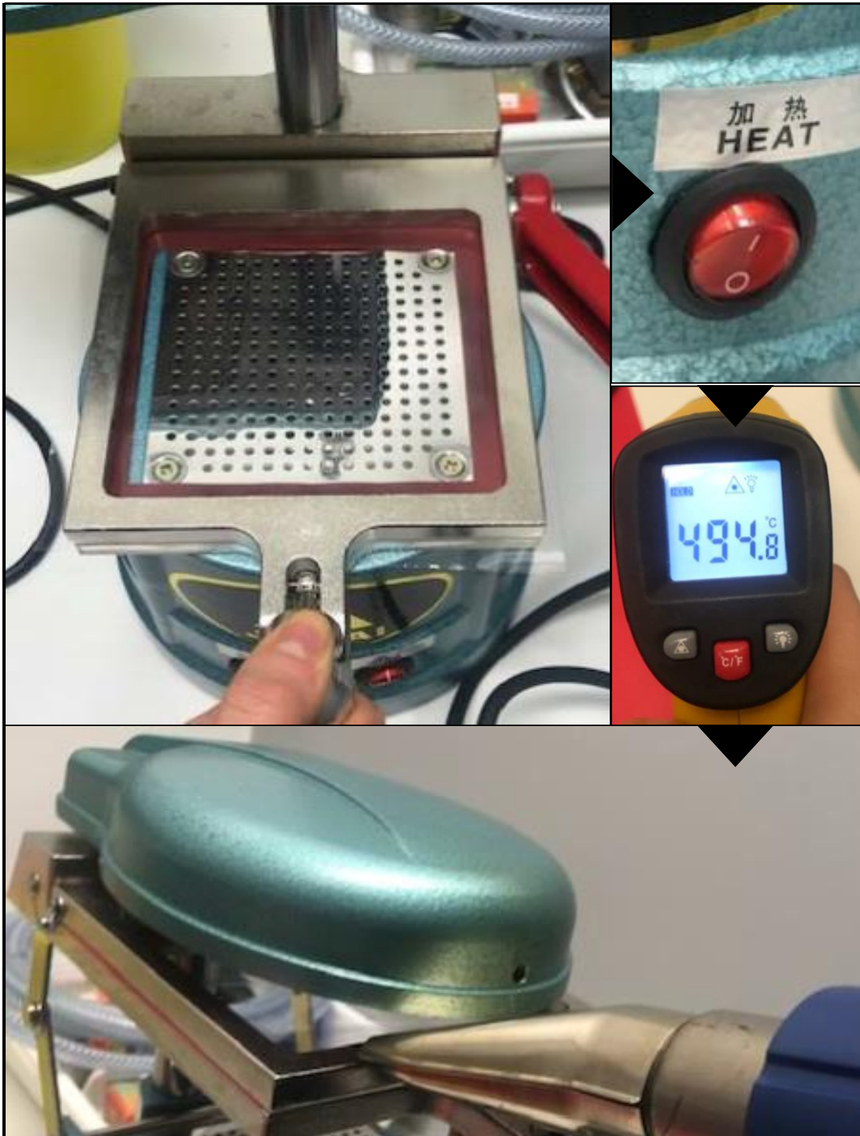
Figure 11: The process of Z1 holder formation. After placing the pre-cut FEP foil into the vacuum-forming machine, the machine should be pre-heated to 480°C to 500°C. Next, the FEP foil is lifted and approached to the heater. The heating process is improved by keeping an industrial dryer close to it manually. The FEP foil is kept in this position to become flexible and start to stretch downwards. This part takes for ca. 30 sec. (the images are modified from Louise Breideband protocol).
