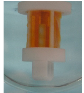
Fig. 2: Photograph of the dispersion releaser filled with nanoparticles loaded with orange dye.
