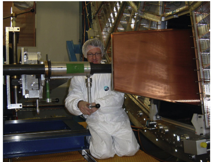
Fig. 17. Insertion of an OROC through the endplate. The tilt, polar and azimuthal angles of the chambers can be adjusted via handles and a transmission system.
