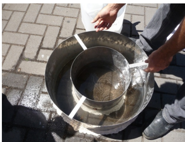
Figure 3. Double ring infiltration test on PICP.
