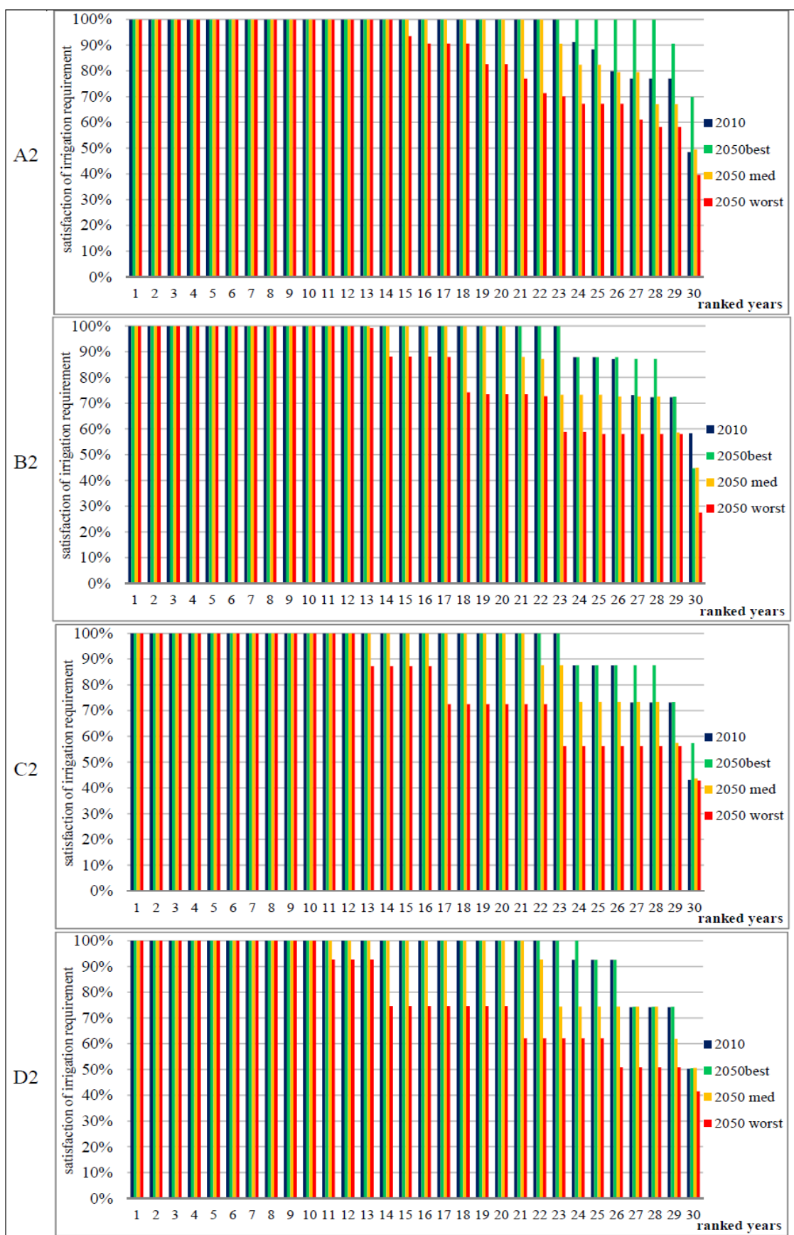
Figure 51: Degree of satisfaction of irrigation water requirement (%) per scenario for two planting seasons under present and 3 future climate scenarios with the gardening size as under present climate. Years are ranked, ending with the driest year.
