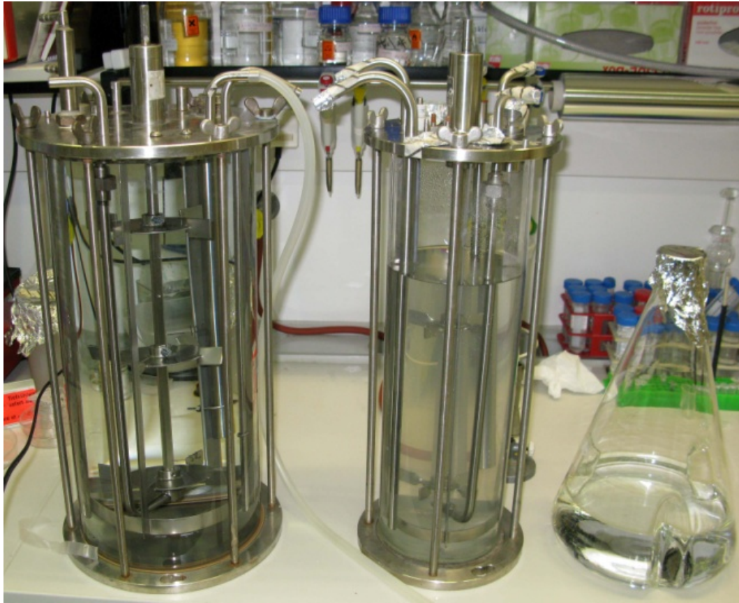
Figure 3.1 Three different liquid culture vessels for C. elegans breeding. The different containers were used for large scale breeding of nematodes. The first reactor could hold up to 10 L of S medium, the smaller contained up to 6 L and the 5 L flask could be filled with up to 2 L medium.
