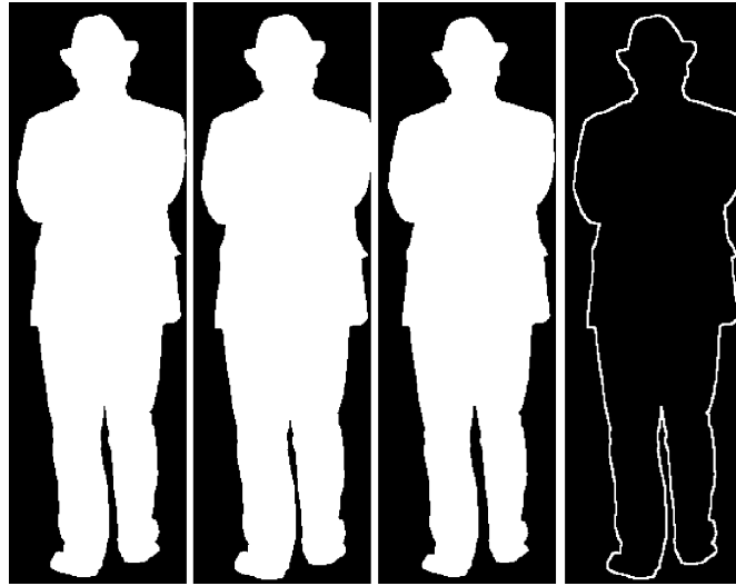
Figure 4.6: Looking from left to right, the first image visualizes the binary instance segmentation mask of a pedestrian bounding box. The second and third images visualize the dilated and eroded versions of the binary instance segmentation mask. The fourth image depicts the boundary mask, which is the result of subtracting the eroded version from the dilated version of the binary instance segmentation mask.
