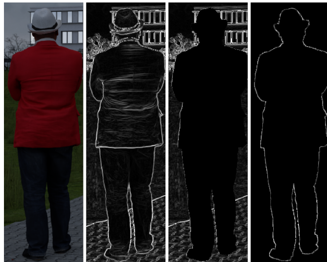
Figure 4.7: Looking from left to right, the first image illustrates a pedestrian bounding box. The second image visualizes the corresponding magnitude vector M . The third image shows the magnitude vector M after it has been filtered by the dilated instance segmentation mask, resulting in the magnitude vector of the background. Applying the boundary mask to the initial magnitude vector yields the fourth and final image.
