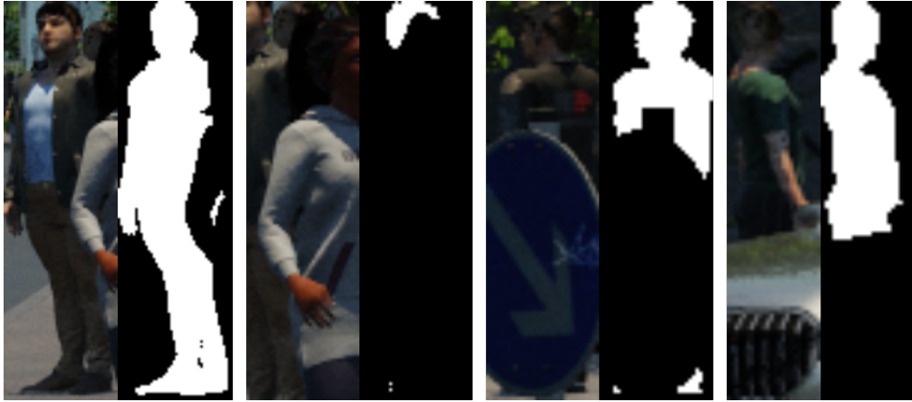
Figure 5.2: Several examples of pedestrian bounding boxes and their binary instance segmentation masks taken from KI-A . Looking from left to right, the occlusion ratios of the four pedestrian instances have been approximated by the occlusion estimation model to be 0.12, 0.86, 0.5, and 0.43, respectively. The ground truth occlusion ratios for these instances are 0.22, 0.95, 0.68, and 0.38, respectively.
