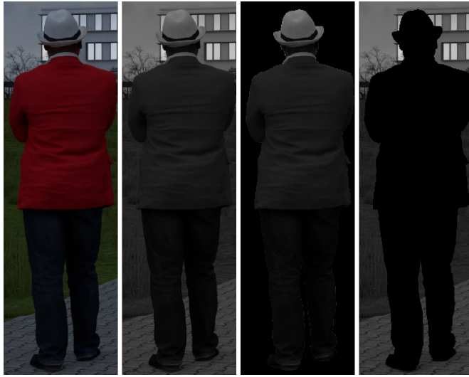
Figure 4.8: Looking from left to right, the first image features a pedestrian bounding box. The second image features a grayscale version of the first image. The third and fourth images visualize the foreground and background of the grayscale pedestrian bounding box.
