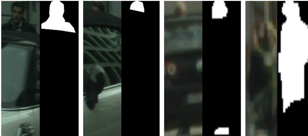
Figure 5.3: Several examples of pedestrian bounding boxes and their binary instance segmentation masks taken from CityPersons . Looking from left to right, the occlusion ratios of the four pedestrian instances have been approximated by the occlusion estimation regression model to be 0.84, 0.99, 0.82, and 0.25, respectively.
