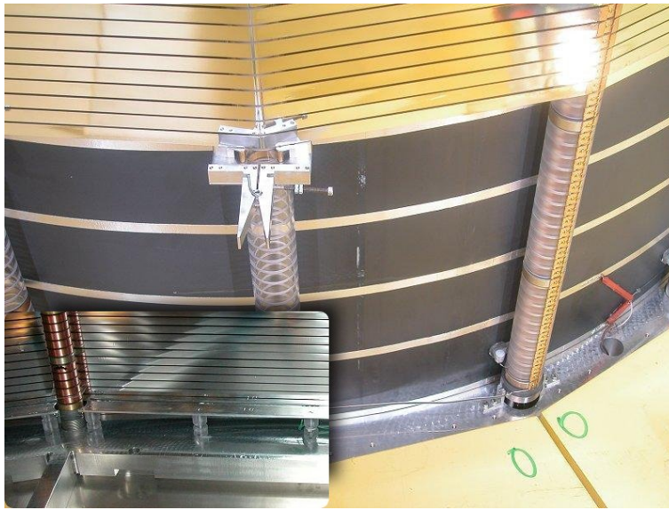
Figure 3.10: Picture of the inner field cage rods, field strips and inner containment vessel with guard rings. The inset shows field strips of the outer field cage and the skirts between the rods.
