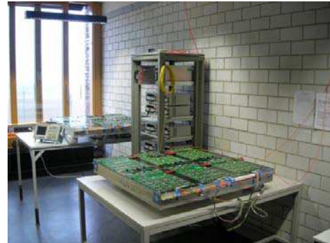
Figure 1: Electronic test stands for the ALICE TRD chambers with pulser and low voltage support.
