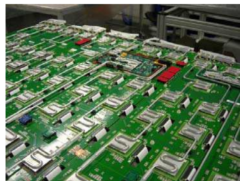
Figure 1: Electronic test stands for the ALICE TRD chambers with pulser and low voltage support.
