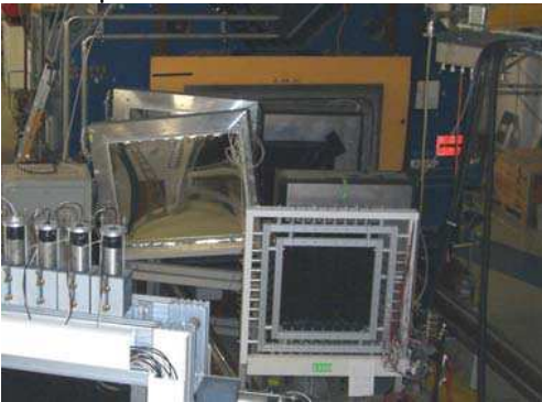
Figure 1: View of DCH installed behind ALADIN in Cave C. The detectors are inclined with respect to each other to avoid ambiguities in tracking.
