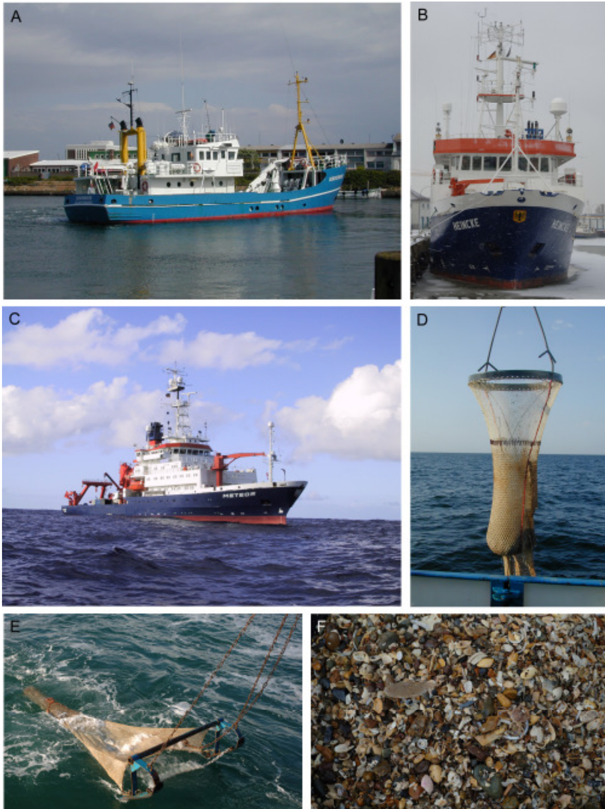
Figure 2.1. Fieldwork in the North Sea. (A) RV SENCKENBERG (length: 36 m) on the coast of the Island Helgoland in the German Bight. (B) RV HEINCKE (55 m) was used for the Dogger Bank winter cruise (North Sea). (C) RV METEOR (97.5 m). (D) Ring dredge (90 cm). (E) 2 m - Beam trawl. (F) Typical benthic sample from the Dogger Bank. Photographs: C. Becker (A, D, E), S. Tränkner (B, F), P. Wintersteller (C).
