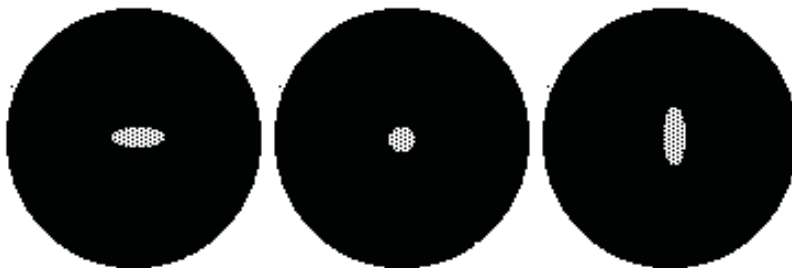
Figure A.3: Astigmatism aberration, from left to right : inside focus (sagittal), best focus, outside focus (tangential).
