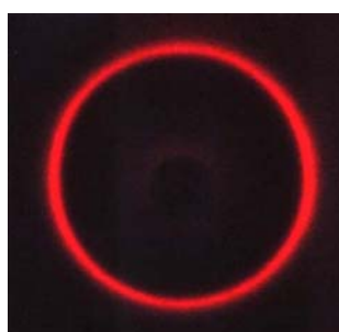
Figure 22 Cone of the surface plasmon coupled directional fluorescence emission of the fluorophores at the surface of the thin metallic film. (taken from [188])
