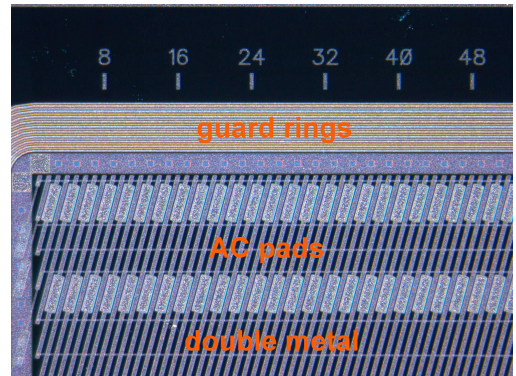
Figure 4.18: P-side of CBM01 full-size sensor with one row of AC pads and 10 guard rings.
