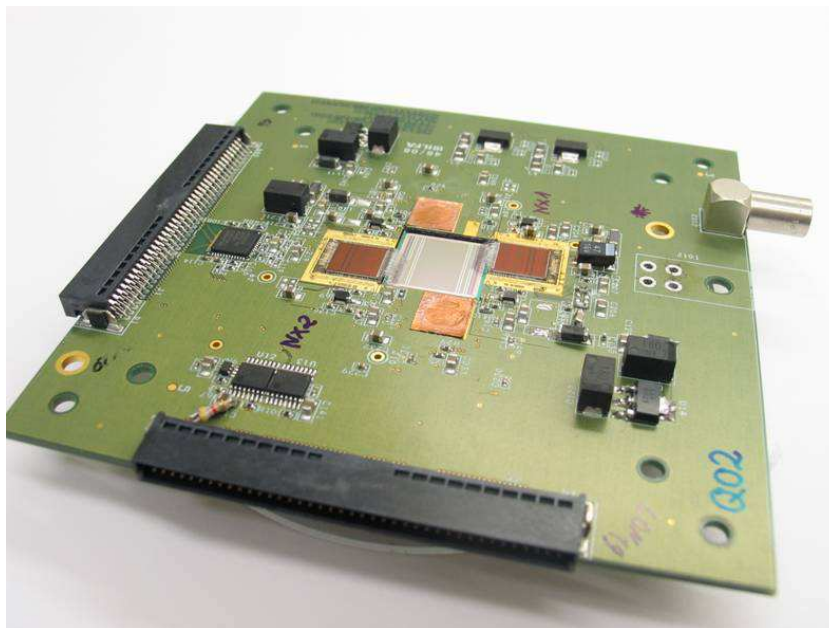
Figure 6.1: A beam tracker board comprising a double-sided CBM02B2 prototype detector wire-bonded to four n-XYTER readout chips, two per side.
