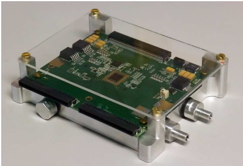
Figure 4.32: n-XYTER front-end board (revision D) mounted on the cooling block for temperature stabilization.
