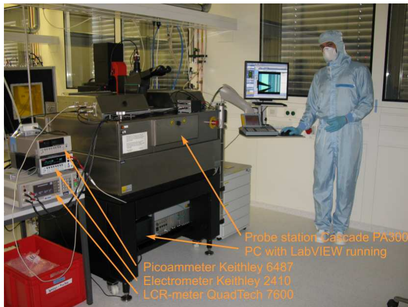
Figure 5.1: Laboratory infrastructure for microstrip sensor characterization in the clean room including shielded probe station, picoamperemeter, electrometer, LCR-meter and an instructed operator.
