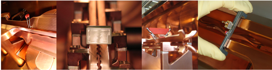
Figure 4.18: Different kind of perturbation capacitors and a ceramic perturbation for the measurement of the field flatness.
