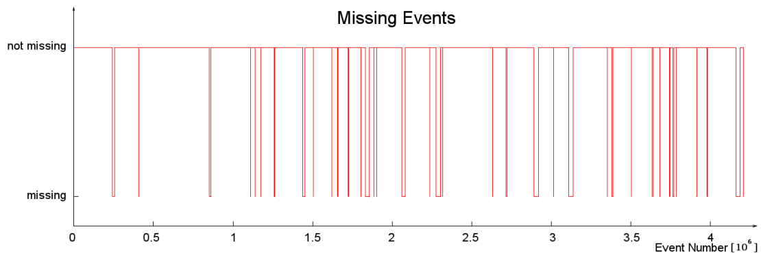
Figure 6.8: During the high data rate run, 5.1 % of the events were lost. The network bandwidth has been near the limit and the event builder has discarded some events due to missing UDP packets.
