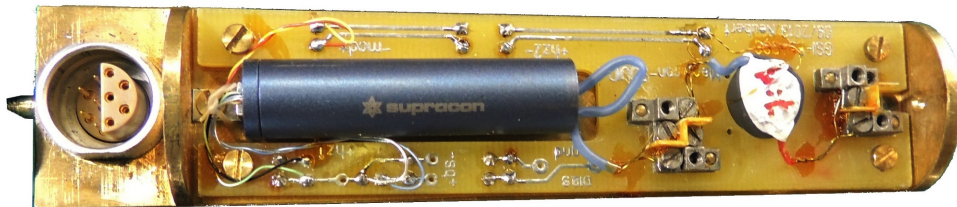
Figure 3.6: Photograph of the dc SQUID sensor ‘CP2S Blue’ mounted on the PCB (shown in blue colour). The matching transformer is shown at right hand side to the SQUID sensor (in white). The 10 pin “lemo type” connector which connect the SQUID cartridge to the FLL electronics can be seen in the left hand side.
