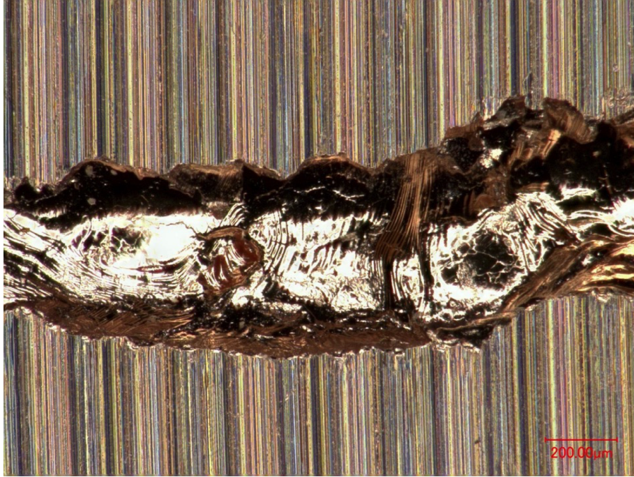
Fig. 6.22: 3D high-resolution picture of hole drilled by the beam in the first cylinder of Target 3. The region between z = 2.4 - 2.6 cm is shown with a magnification of 200x.
