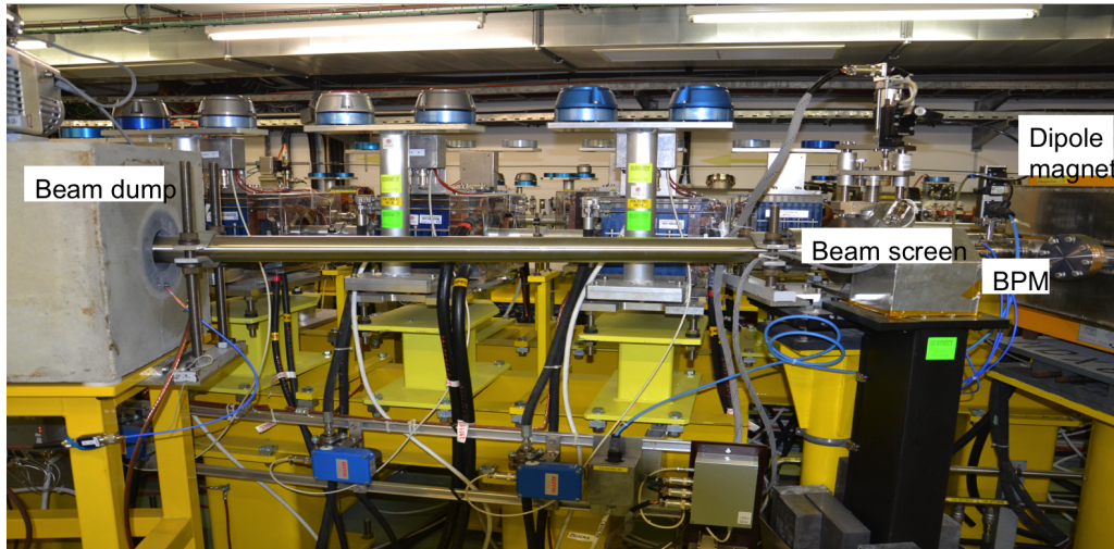
Fig. 9.21: Picture of the beam line before the modification. The kicker magnet to send the beam to beam line is shown on the right, followed by a screen station to monitor the beam profile and position. Further downstream the beam can be dumped on the dump block, which can be additionally used as Faraday-cup for intensity measurements.
