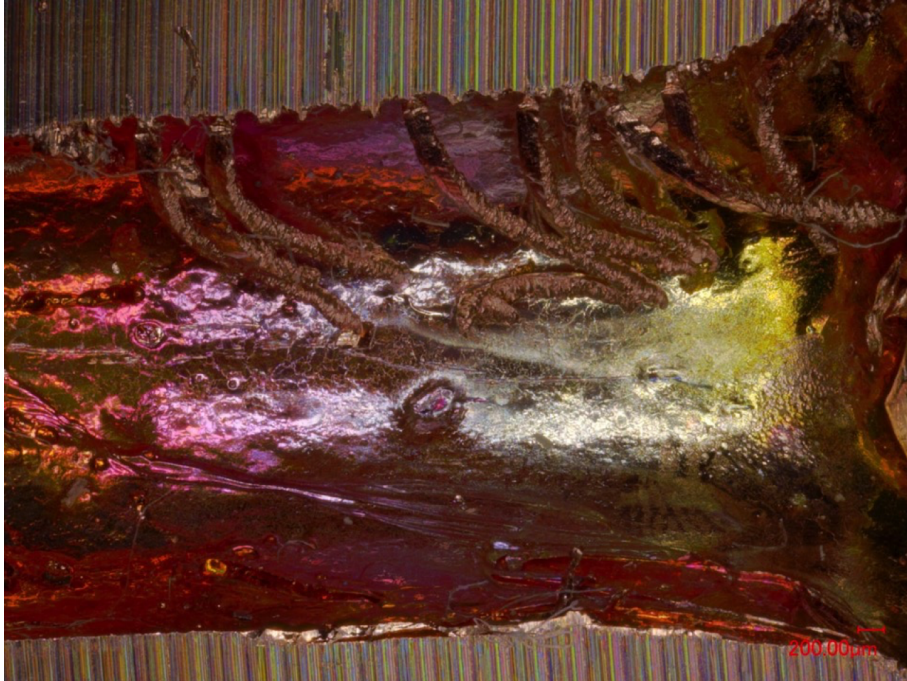
Fig. 6.23: 3D high-resolution picture of hole drilled by the beam in the first cylinder of Target 3. The region between 9.3 - 10 cm is shown with a magnification of 50 x. The coloring is real.
