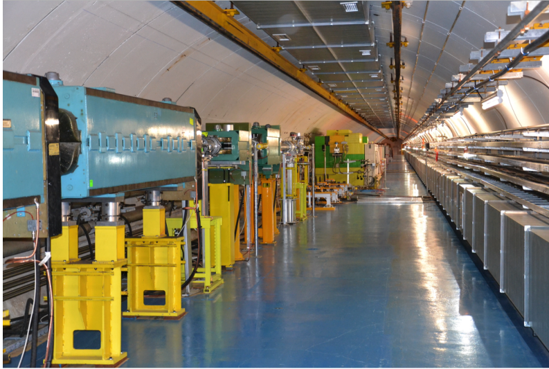
Fig. 4.15: Picture of the HiRadMat tunnel with the last focussing and bending magnets (light blue), the platforms (yellow on the floor) for the experimental tables and the beam dump at the end of the tunnel.
