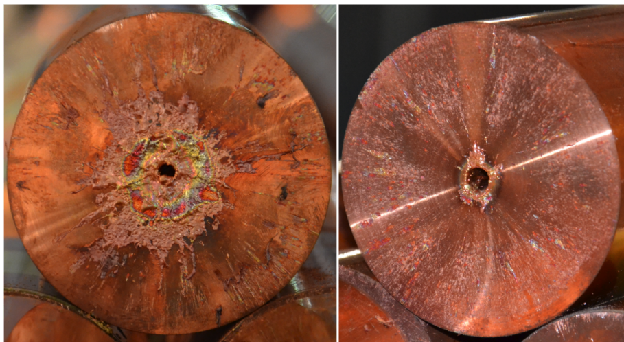
Fig. 6.13: Front (left) and back (right) of the fifth cylinder of target 3. The hole diameter is getting smaller as the energy deposition decreases.
