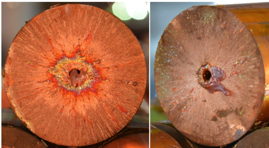
Fig. 6.11: Front (left) and back (right) face of the third cylinder. Molten copper is leaking out of the hole, solidified splashes are clearly visible.
