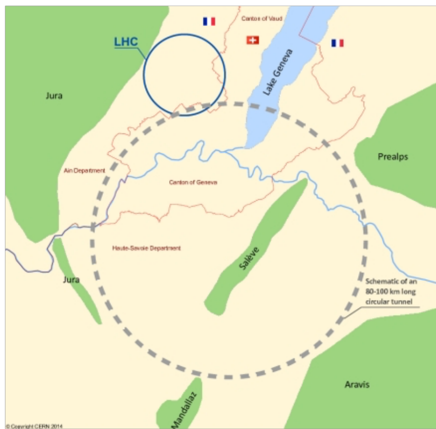
Fig. 2.5: Possible location of the FCC (dashed line). The present LHC is marked in blue. The lake geneva is on the top of the picture.
