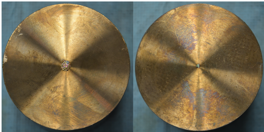
Fig. 6.17: Front (left) and back (right) of the ninth cylinder of target 3. Solidified splashes on the front plate are clearly visible. On the back face a decoloring of the copper on beam axis is visible. No hole detectable from visual inspection.
