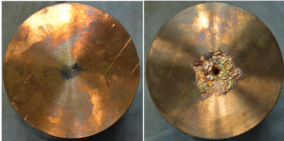
Fig. 6.9: First cylinder of target 3. The beam enters the target on the front plate (left) the surface is damaged, material is ejected towards the aluminum end cap. At the back face of the cylinder (right) a hole is clearly visible, material is ejected towards the front face of cylinder 2. Reflected copper splashes and ejected splashes from cylinder 2 solidified on the surface. The copper in this cylinder was liquid (first half) and in gaseous state (second half).
