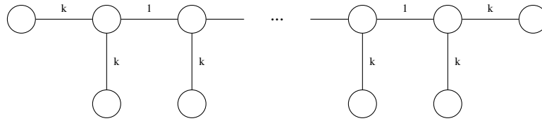
Figure 4.4: A weighted graph as an input where the clustering approach produces an error of \Theta(k) .
