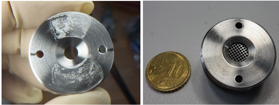
Figure 3.2: Left: old aperture of 4 mm diameter. The contamination on the surface is silver paint that was used as adhesive in order to prevent the coil holder from turning during the assembly of the source. Right: the widened aperture of 8 mm. Here, the filament and the grid have already been assembled.
