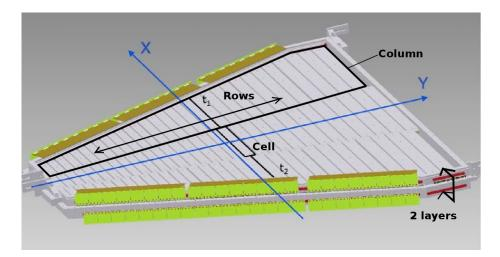
**Figure 2.8:** Technical drawing of one sector of resistive plate chambers covering polar angles from  $18^{\circ}$  to  $45^{\circ}$ . The RPC detector is used for time-of-flight measurements.
