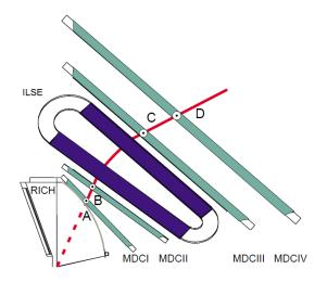
Figure 2.3: Schematic view of the magnetic spectrometer consisting of four planes of mini drift chambers (MDC I-IV) and the superconducting toroidal magnet (ILSE). A charged particle traversing the spectrometer ionizes the gas in the drift chambers. Its trajectory and momentum can be reconstructed via the measured hit points in the MDCs and its deflection caused by the magnetic field  $\vec{B}$  (see 3.5.3).
