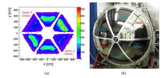
**Figure 3.24:** (a) MDCI hit distribution in the six sectors. The non-uniform distribution with respect to the azimuthal angle can be traced down to different materials used for the RICH sectors (b). The glass mirrors in the RICH detector used for sector 2 and 5 absorb more ( $\delta$ -)electrons resulting in different loads in the drift chambers. Figures taken from [248].
