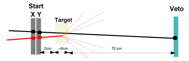
**Figure 2.10:** Scheme of the start and veto system. In the ideal case assuming 100% efficiency of all detectors, a beam particle is inducing a signal in the two modules of the start detector. If a reaction in the target takes place there is no response from the veto detector (red), if not, the beam particle will produce a hit in the veto detector as well (black). The signal in the start detector defines the start time  $t_{coll}$  of the reaction.
