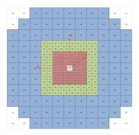
**Figure 2.12:** Front layout of forward hodoscope indicating the scintillator blocks surrounding the beam line [238]. The dimensions of the innermost scintillator blocks (red) are  $4 \times 4 \text{ cm}^2$ , followed by  $8 \times 8 \text{ cm}^2$  (green) and  $16 \times 16 \text{ cm}^2$  (blue) for the outermost cells.
