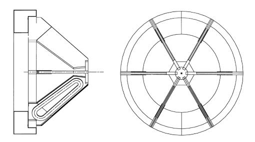
**Figure 2.6:** Technical drawing of the ironless, superconducting toroidal electromagnet ILSE, (left) side and (right) front view.
