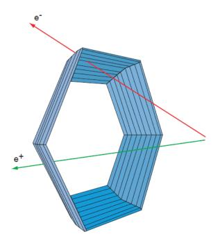
**Figure 2.7:** Schematic design of scintillator array of the time-of-flight wall TOF, covering polar angles from  $44^{\circ}$  to  $88^{\circ}$ .
