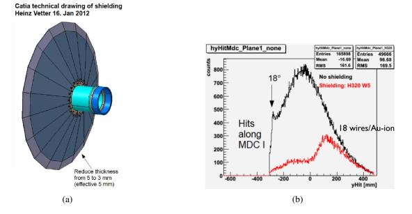
**Figure 3.22:** (a) Technical drawing of the  $\delta$ -electron shield which was installed in 2011/12 behind the target. (b) Simulated hit distribution as a function of y detector coordinate in innermost drift chamber plane MDCI with and without shielding. A clear reduction of the load in the low theta region (corresponding to low y) is obtained when introducing the  $\delta$ -electron shield. Figures taken from [254].
