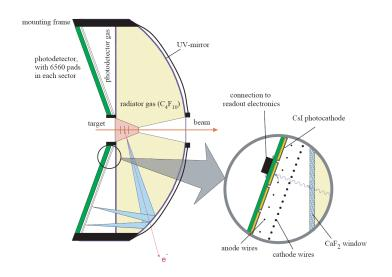
**Figure 2.13:** Schematic cross section of the RICH detector indicating the emitted Cherenkov light (blue areas) reflected on a UV-mirror and detected by a CsI photocathode.
