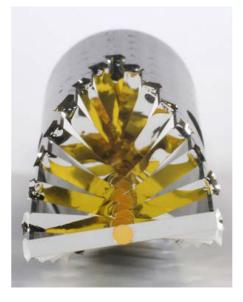
One of the main requirements for the design of the target is to keep the conversion from  $\gamma$  radiation inside the target material into  $e^+-e^-$  pairs as low as possible, which is the reason for the segmentation. By maximizing the distance the contribution of conversion in the following segments can be neglected since the  $\gamma$  radiation typically leaves the target material with large
