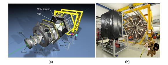
**Figure 2.1:** (a) Exploded view of the HADES setup. Indicated are the Mini-Drift Chambers (MDC) together with the superconducting magnet (ILSE) used for track reconstruction of charged particles, the Ring Imaging Cherenkov (RICH) and Pre-Shower detector for lepton identification as well as the RPC and TOF providing time-of-flight measurements. (b) Photograph of the backside of the detector in operational mode including the Forward wall.
