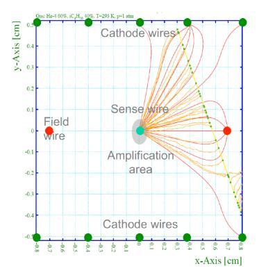
Figure 2.5: Schematic view of a charged particle traversing one MDC cell. A charged particle ionizes gas molecules statistically along its trajectory (green dots). The primary electrons are accelerated towards the anode wire (red lines) initiating an avalanche of secondary electrons few  $\mu$ m above the sense wire (gray area), inducing a signal [235].
