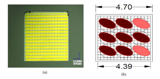
**Figure 2.9:** (a) Front view of the multi-strip start detector (module 1) showing the 16 monocrystalline diamond-based stripes. (b) During the Au+Au beam time the start detector was relocated nine times (indicated by the black rings) in order to minimize performance losses due to radiation damage. During one spill the beam is wandering within one ellipse.
