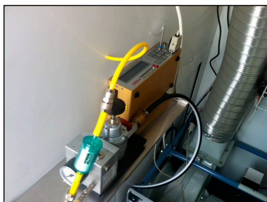
Figure 3. Aerosol spectrometer (yellow box) and pressure regulator with pressure indicator of the VKL mini. The dilution system VKL mini attenuates the sampled air in a ratio of 1:10 with neutral compressed air.
