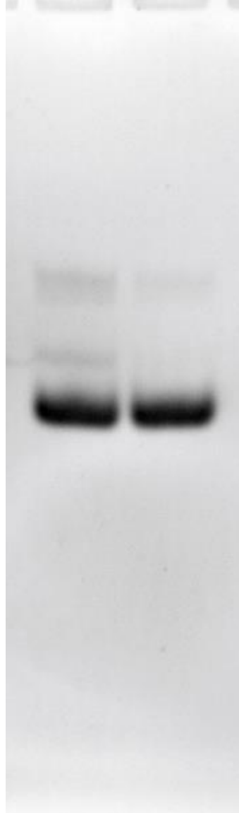
Figure S1. Native polyacrylamide gel electrophoresis (PAGE) assay performed in order to confirm purity of the RNA after purification. An 8% polyacrylamide (PAA) gel was used with 650 \mu\text{g} of RNA. Two purified transcription products from separate preparations are shown; the product on the right was used for all MAS DNP experiments in this work. No marker was used.
