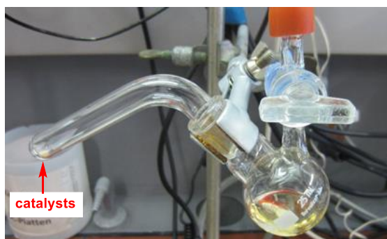
Figure S1. Apparatus used for the preparation of ester 11 . Through turning the bent tube the catalysts are brought to the degassed solution of 4-iodo-PyMTA ethyl ester 9 and 4-ethynyl-PyMTA ethyl ester 10 without opening the apparatus.
