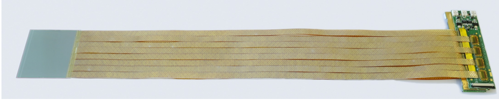
Figure 1.16: Module assembly: 1024 sensor channels of 62 \times 62 \text{ mm}^2 sensor connected via 50 cm long micro-cables to 16 ASICs placed on two FEBs (frond-end-board) for the p- and n-side.
