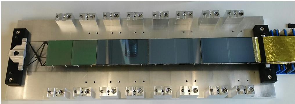
Figure 1.17: Example of the ladder made of carbon fiber and sensors attached to it: two of 62 \times 62 \text{ mm}^2 and three sensors of 62 \times 122 \text{ mm}^2 size. Microstrip cables are placed underneath.
