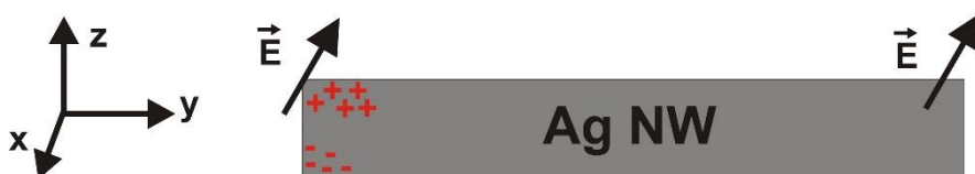
Figure S4. Although the nanowire is symmetrical, due to the incident light the excitation at both ends differs resulting in a much stronger SPP excitation here at the left side. The E-field (oscillating in the yz-plane) can move electrons in both directions as it “sees” the entire front facet; on the right side it is “shadowed” by the nanowire itself.
