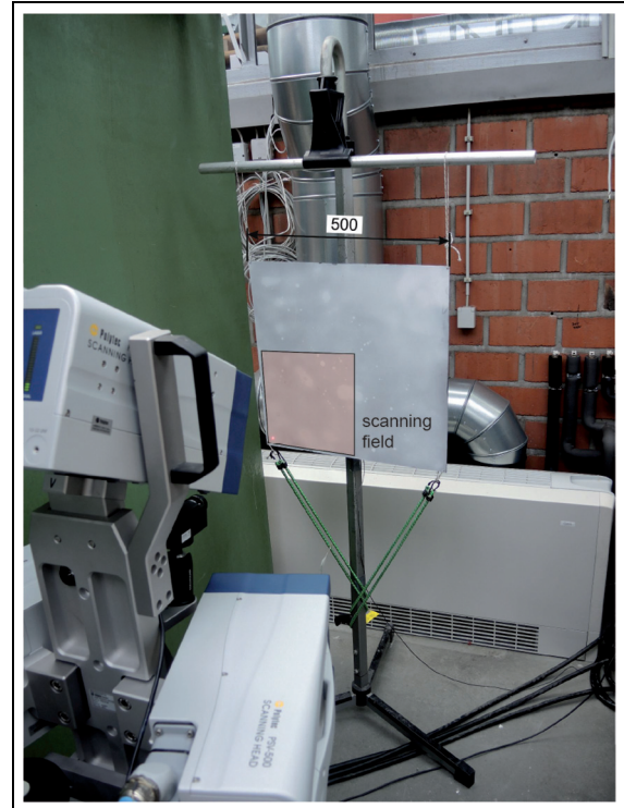
Figure 8. Experimental setup with the scanning laser Doppler vibrometer and the “wave field plate.”
