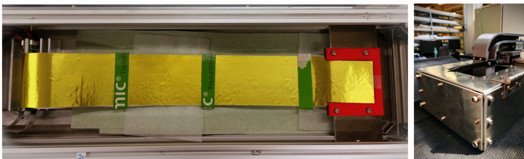
Figure 6.14: Pictures of the module test box showing a module under test. The 3D printed sensor holder can be seen in red.
