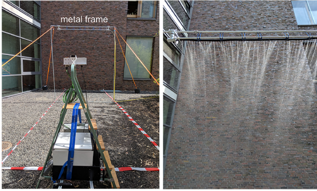
Fig. 2. (Left) Photo of the experimental setup. Water is sprayed from the metal frame toward and away from the radar at different angles. (Right) Rain distribution.
