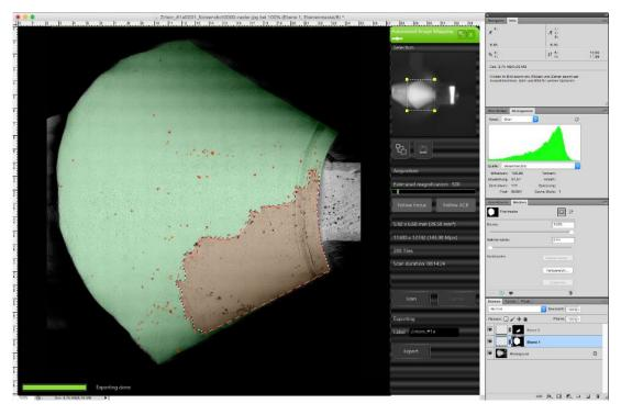
**Figure 3.** Computerized planimetric calculation of the proportion between area covered with contaminants (red) and the total surface of the abutment shoulder displayed (green).
