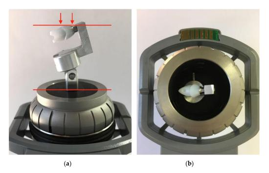
**Figure 2.** Test set-up: (**a**) Customized device and tilting turntable for exactly reproducible positioning of specimens during SEM; (**b**) specimen after lowering to optimum working distance.
