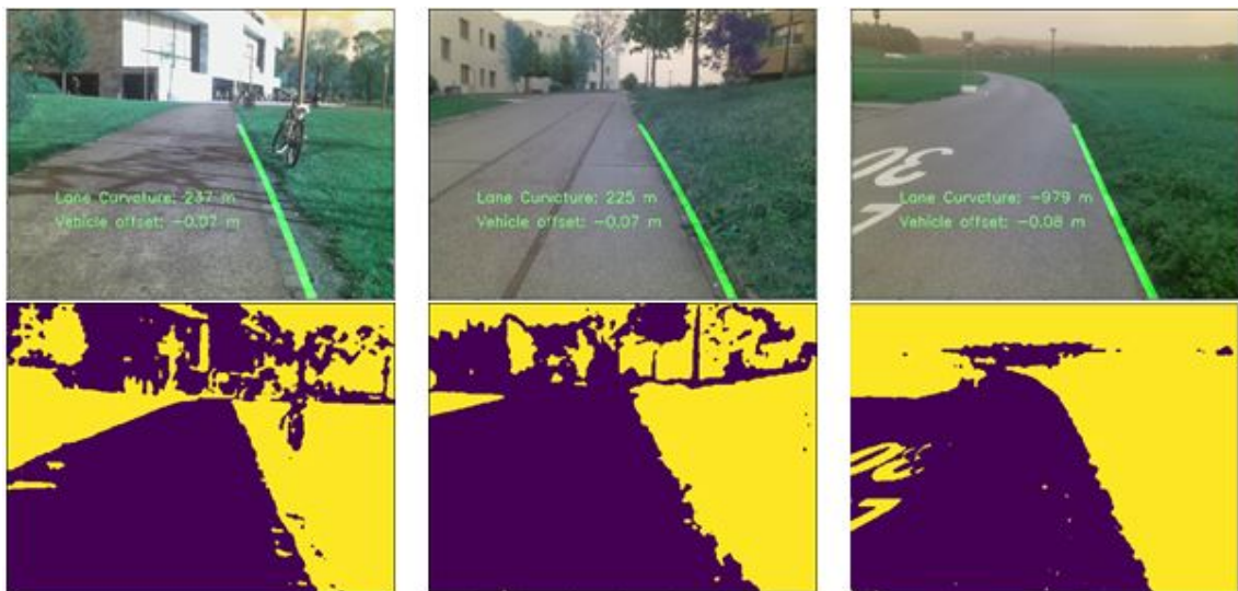
Figure 4.2: Straight road detection
