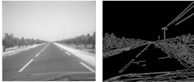
Figure 2.6: Canny edge detector example (right) original image (left) [28, p. 205]
