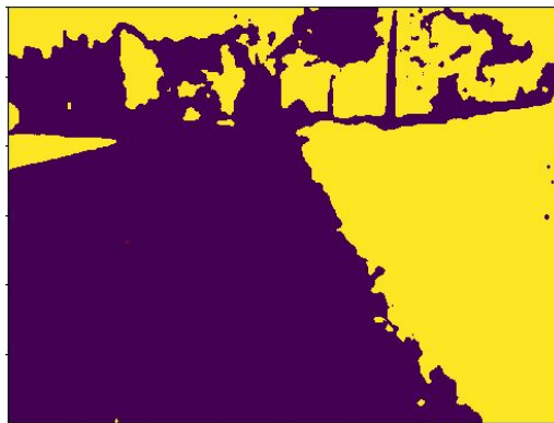
Figure 3.8: Roadside detection on straight street without lanes
