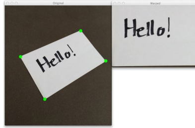
Figure 2.5: Example of a perspective transformation [64]
