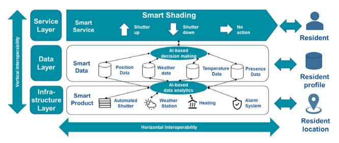
Fig. 1: ForeSight's layer-based architecture to enable horizontal and vertical interoperability for reducing almost all vendor- or companyspecific dependencies, here shown by the example of a smart shading use case.
