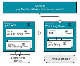
**Fig. 2:** ForeSight platform approach considering different smart home middleware systems, here openHAB, which interacts with a WoT technology stack. On top of these technologies companies create and connect their services as providers.
